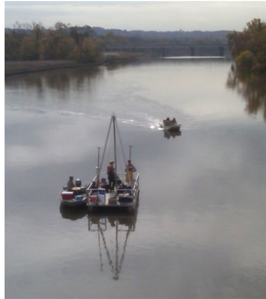
Boat-mounted drilling equipment was used to collect sediment samples from the bottom of the Anacostia River.
